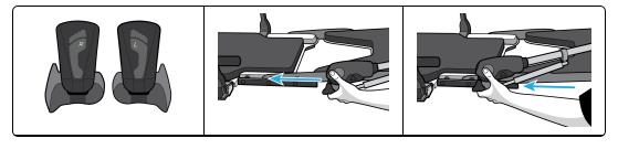
3. Tighten rail knobs by turning clockwise.
