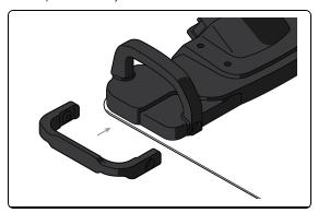
Reinstall screws to secure handle and rail. Tighten screws until handle and rail are securely attached
