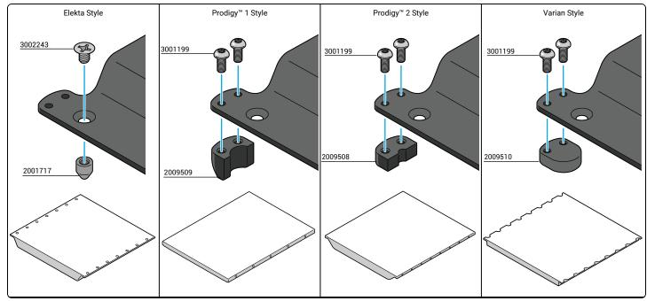
2. Tighten screws until indexing features are securely attached.
