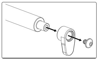
2. Place Dual Width Stabilization clips and use Allen wrench to secure.
