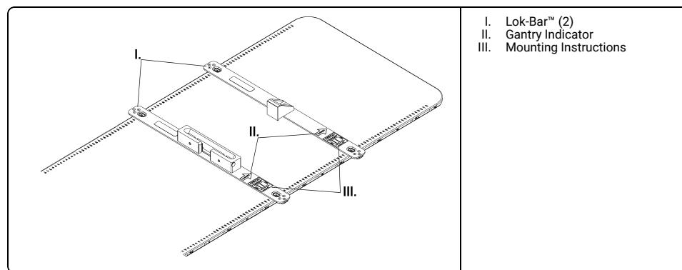
2. Place Varian MPC IsoCal phantom mount onto each Lok-Bar™.
