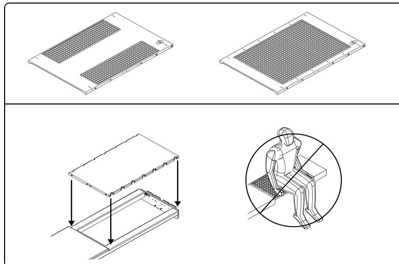
2. Ensure that the orientation is correct and securely attached.
