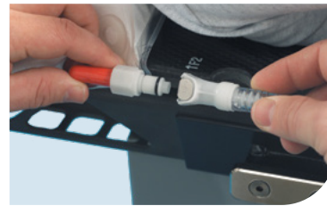
Self-sealing quick-release valve
